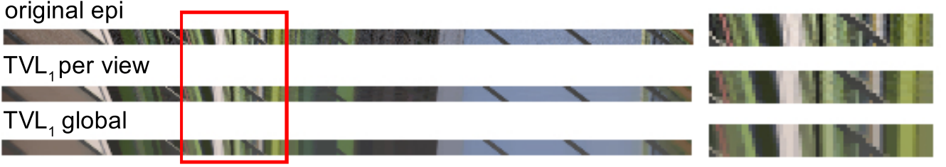
Figure 2: Visualization of the horizontal epi view for the red scanline in Figure 3 (a). From top to bottom: the epi from the original light field; the epi after applying TVL_1 filter to each view separately; the same epi after applying a 4D TVL_1 filter to the whole light field volume using our approach. We can observe (by zooming in the digital version), areas with very similar colors are flattened, while sharp discontinuities are preserved, effectively removing noise and promoting angular coherence.
